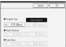
**7** Check the value of Scan Area (X3) and [Auto Detect] are displayed, and then press [OK].
